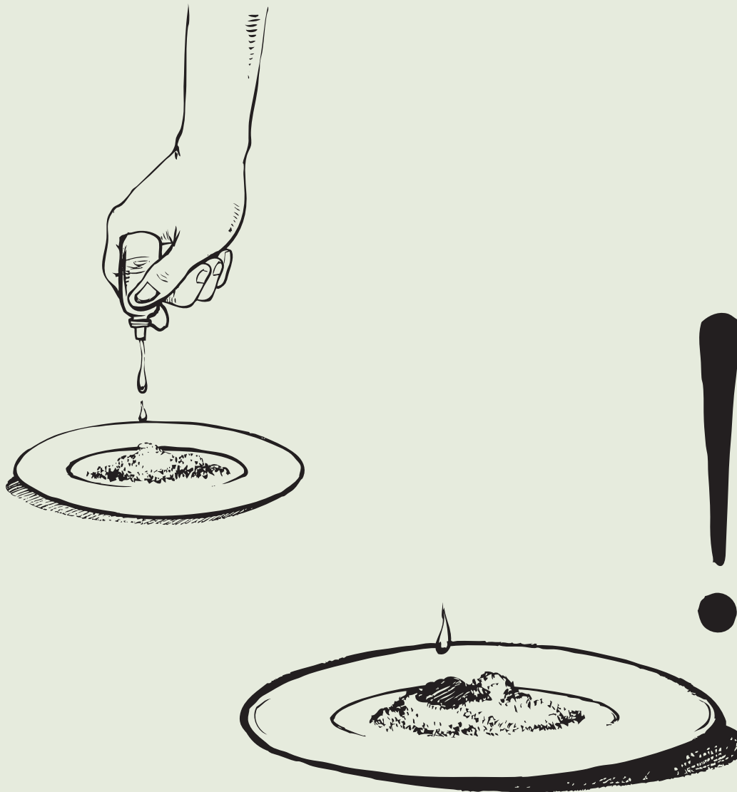
Positive result of iodine test –salt turns orange or red
